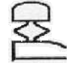
MG - 7a forms the hinge side of a seal / gasket, where the other three sides use MG - 7
